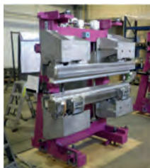
Revolver Mobile Undulator Carriages for the E.S.R.F. in France. Repeating Parallelism tolerance between the beams is 0,05 mm over 2,5 meters incl. beam rotation.
