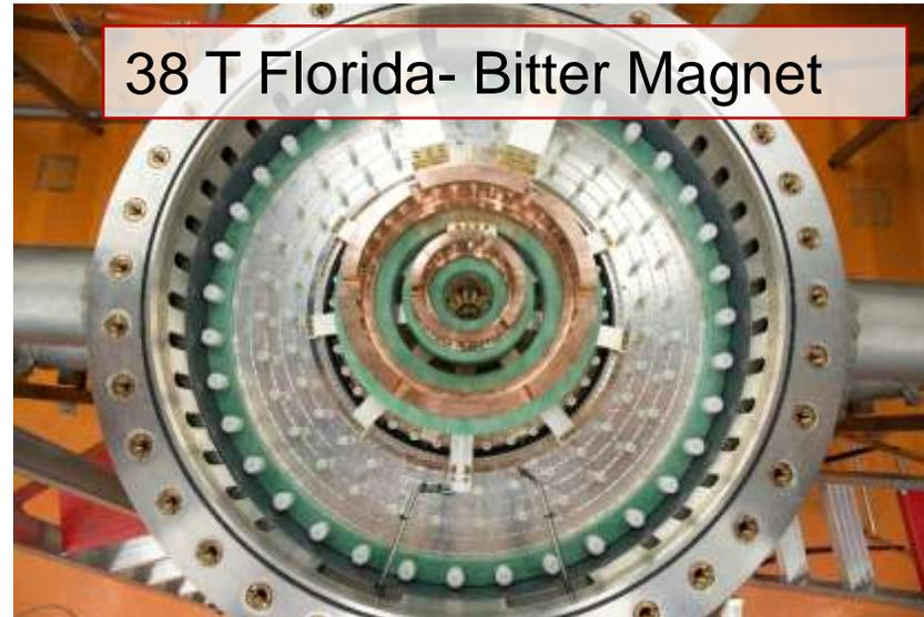
Electrical Power: 22 MW (40 kA, 550 V)
