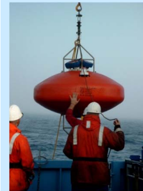
Hydrodynamic shaped buoyancy units
