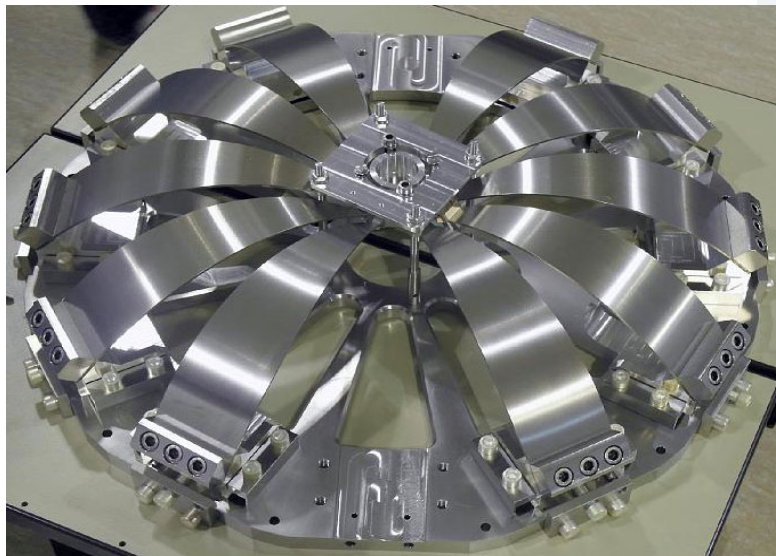
GAS spring Load 420 kg Frequency 200 mHz
