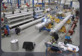
Project scope included thermal design, engineering, manufacturing, and supply of feed caps, tunnel transfer lines and surface transfer lines for the LCLS II project.
