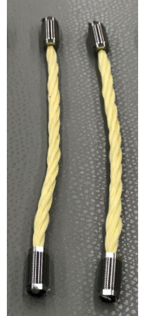
T0-T2 Superconducting Nb flex cable trial Courtesy: Hightec and University of Geneva
