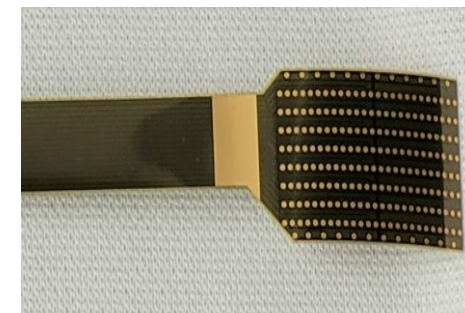
T0-T2 Superconducting Nb flex cable trial Courtesy: Hightec and University of Geneva
