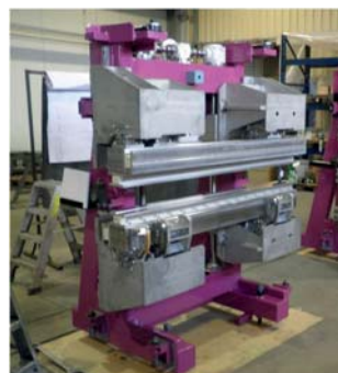
Revolver Mobile Undulator Carriages for the E.S.R.F. in France. Repeating Paralellism tolerance between the beams is 0,05 mm over 2,5 meters incl. beam rotation.
