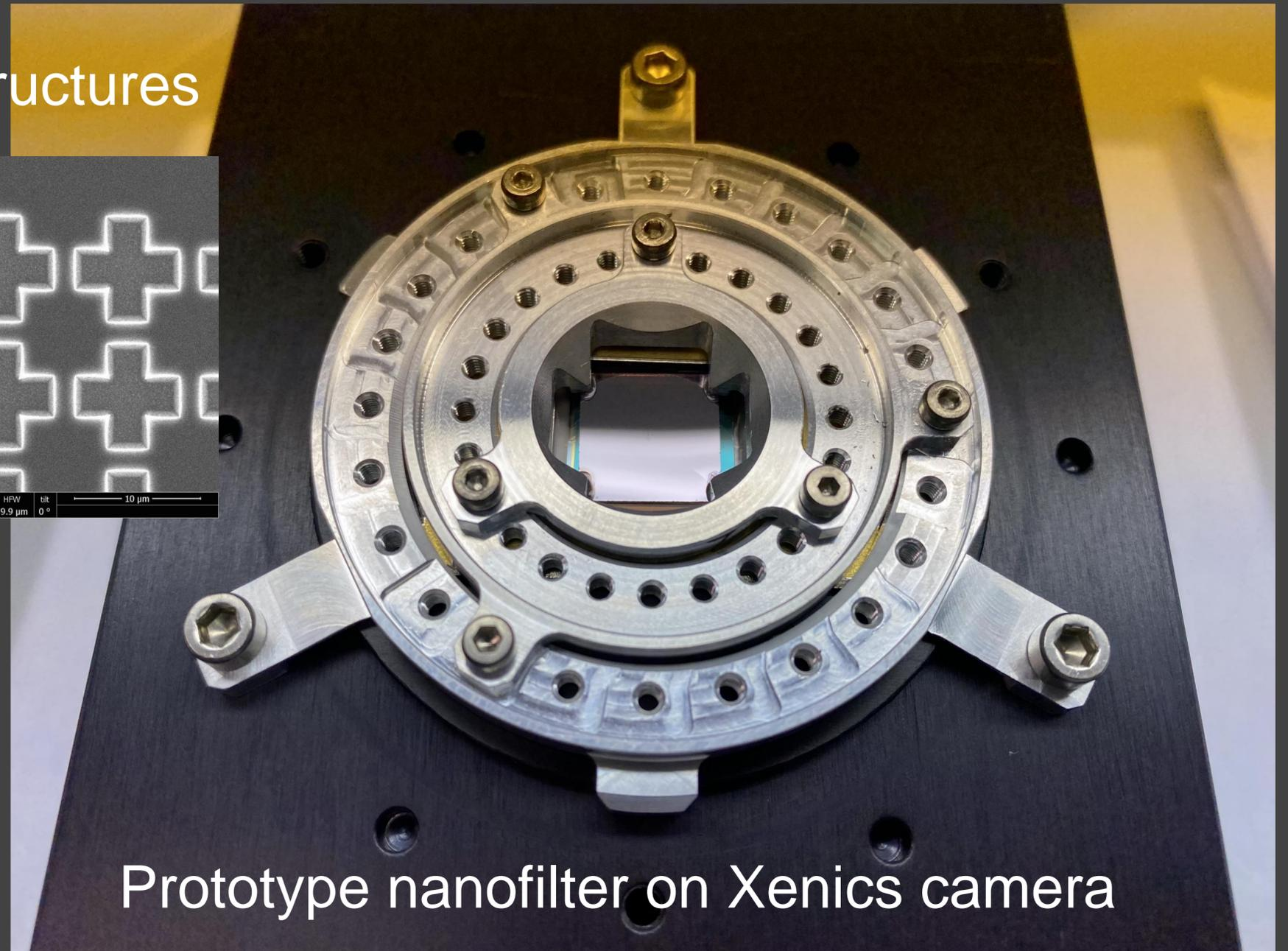
Goal: ultra-compact imaging spectrometers measuring trace gases
