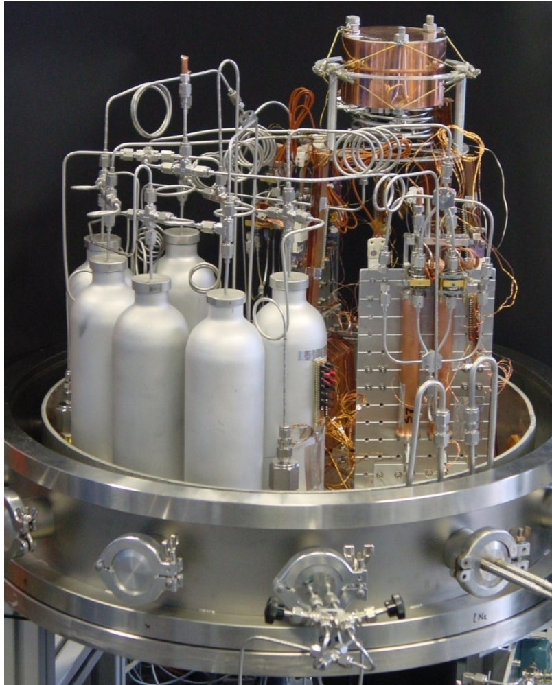
Helium sorption-based cooler 50 K to 4 K (precooled at 14.5 K)
