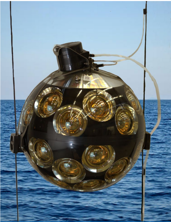
1 optical module = 31 photomultiplier tubes
